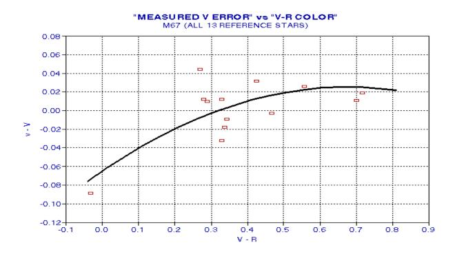
Figure 27 - Dependence of measured "v" magnitude error on V-R color for the "8E/Schuler" system and based on all 13 M67 comparisons stars.
